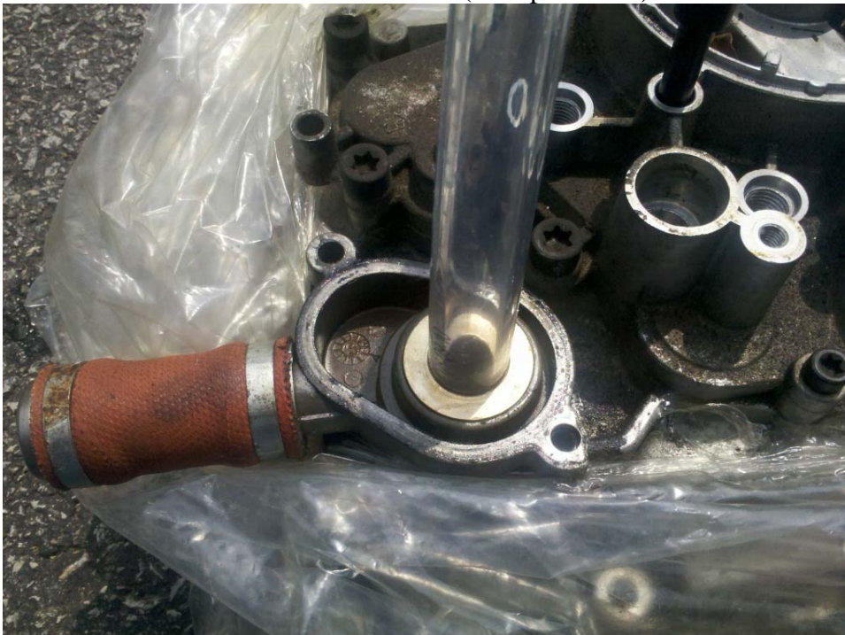
Fig 7.1.3 Adapter fits snugly into the oil cooler coolant outlet port
