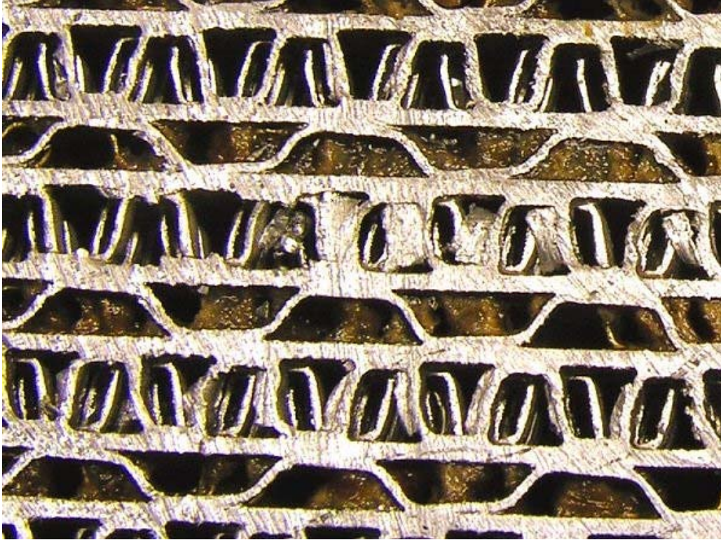
Fig. 3.1 – Plugged oil cooler taken from a 2003 6.0 with 101,000 miles.
