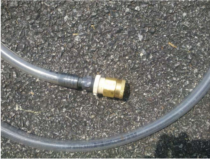
fig 7.1.1 Oil cooler flush adapter
