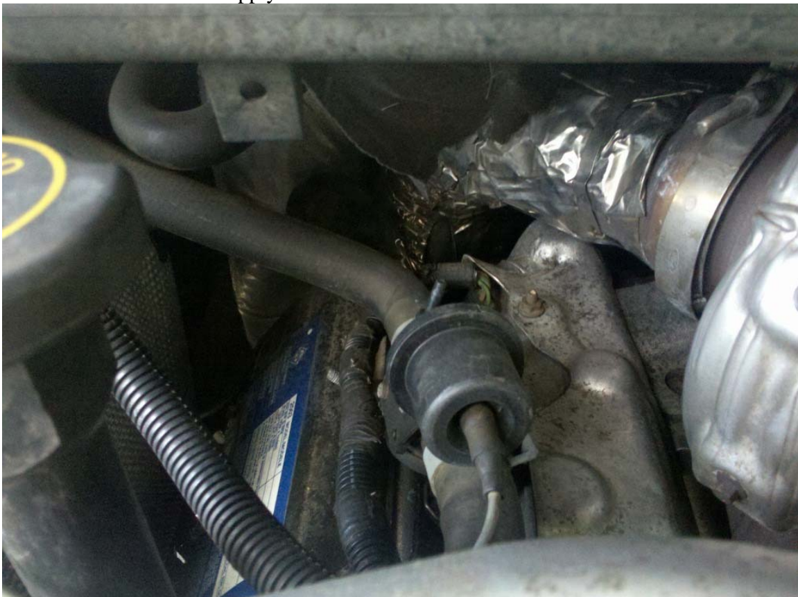
Fig 7.2.1 Heater control valve. Disconnect hose closest to the firewall of the vehicle
