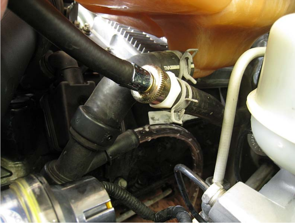
Fig 7.2.1 Adapter inserted in heater core return line at bottom of degas bottle.
