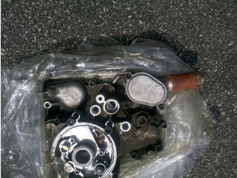
fig 7.1.2 Oil cooler removed from engine
