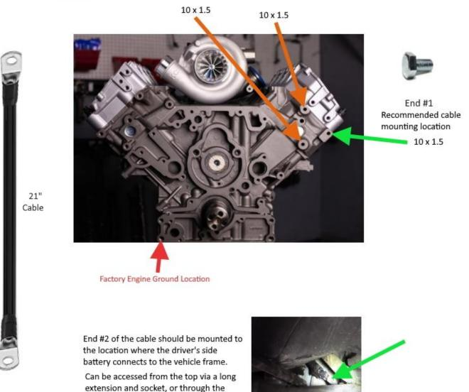
\*\*\* We recommend using a thin film of conductive No-Ox ID coating on all positive and negative battery cable connections. Why? Even 50+ year old phone system connections, which were coated with No-Ox at installation, have been reported to show zero signs of rust, oxidation, or corrosion. The stuff works!!
